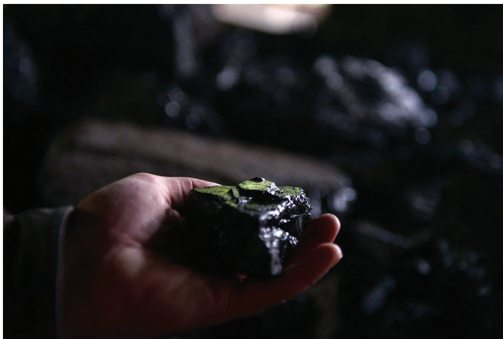
Sub-bituminous coal from RMU Zenica has the highest heating value compared to other coals in BiH. This value can vary from 19,000 to 25,000 KJ/kg, but also has a high sulfur content (2%-6%). In this mine the coal is extracted by shaft mining. (Photo: CIN).
